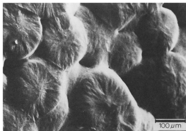
Figure 2 Scanning electron micrograph of PBFP spherulites cast from the concentration THF solution at room temperature. Specimens were sputtered with Au in an argon atmosphere at 10^{-2} Torr. Micrograph was taken at 15 Kv
