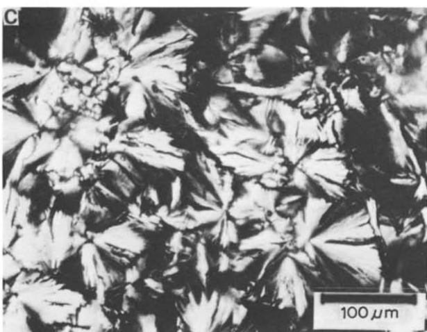
Figure 12 Morphological forms obtained after melting PBFP at 250 °C (5 min) followed by isothermal crystallization at 231 °C, quenching in liquid nitrogen and then reheating to room temperature. Some illustrated morphologies are: (a) negatively birefringent spherulites; (b) aggregated crystals; (c) crystalline spherulitic aggregates
